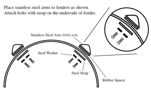
Mount fender to truck's chassis as shown by using 3/4" inch fine pitch threaded bolts provided.
